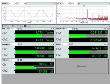
Test conditions: -5dB sinusoidal signal, 20Hz-20kHz, RCA line output (10kΩ load)
