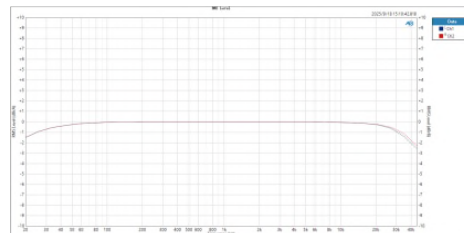
Test conditions: -5dB sinusoidal signal, 20Hz-20kHz, XLR3 balanced line output (10kΩ load)
